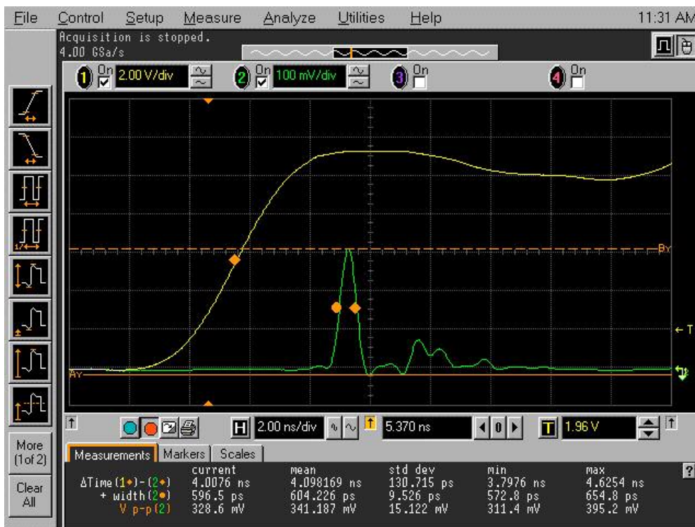
Figure (1) Oscilloscope record showing the relative timing of the voltage waveform (yellow) applied to open the Q-switch and the laser output pulse (green) in a miniature laser experiment. For these traces the temporal resolution is limited by the finite bandwidth of the diagnostic system.
