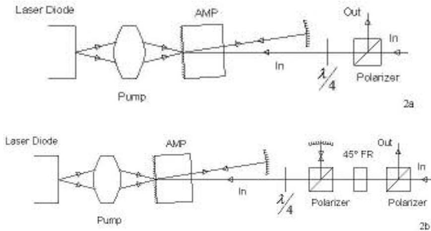
**Fig (2).** Two simple arrangements that provide multi-pass ( $M > 2$ ) amplification. In Fig (2a)  $M = 4$ , and in Fig (2b)  $M = 8$ .
