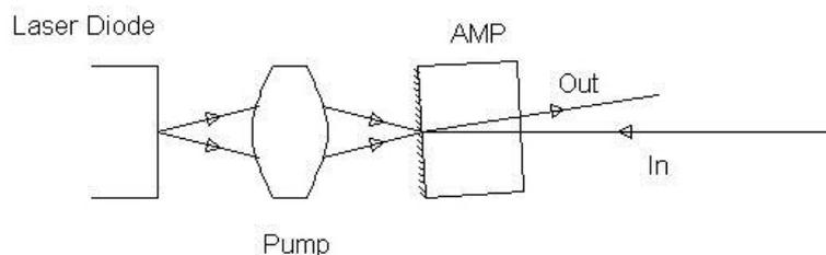
**Fig (1)** Simple arrangement for double-pass operation of an end-pumped SSL amplifier
