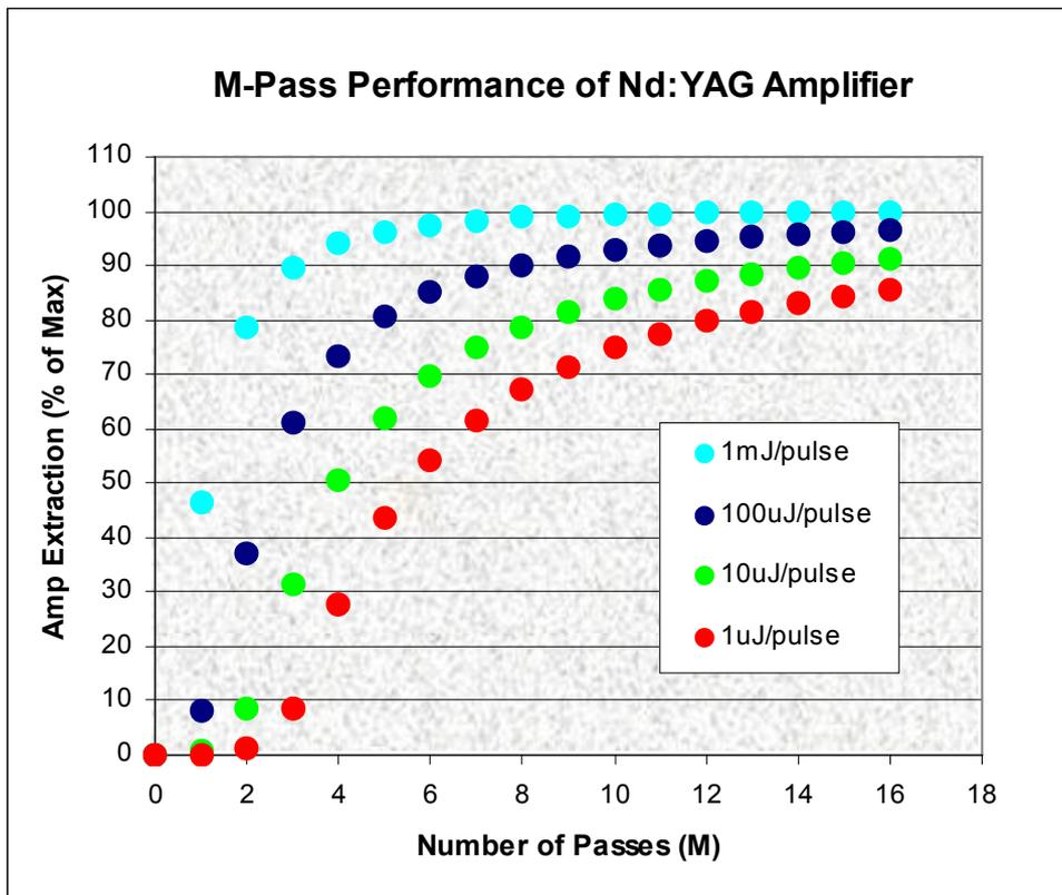
**Fig (3)** Multi-pass Nd:YAG amplifier with beam overlap and input pulses of  $1\mu\text{J}$  to  $1\text{mJ}$  at low rep-rate
