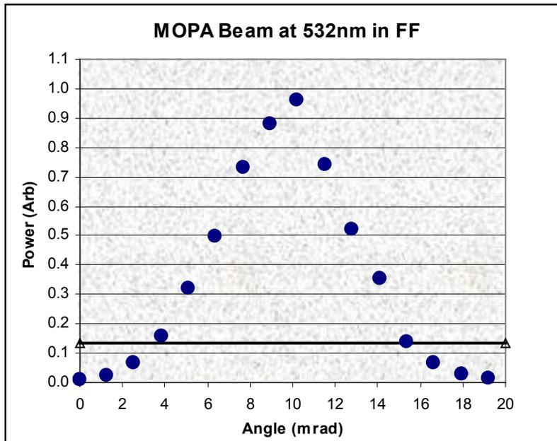
**Figure (3)** Far-field 532nm beam from the KTP doubling crystal at 250kHz. In this example, the MOPA was operated at ~ 1500mW and produced ~ 475mW at 532nm in ~ 3.1ns pulses.
